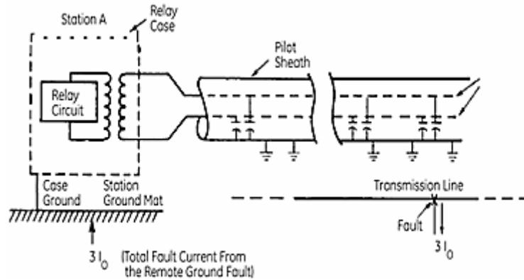
Fig 5. - Station mat .ground potential rise
