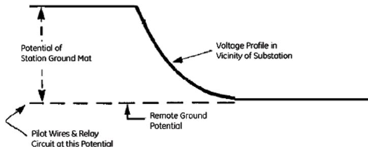
Fig 6. Typical Ground Potential Profile During SLG Fault
