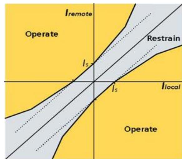
Fig. 1 Differential Protection Operating Characteristic
